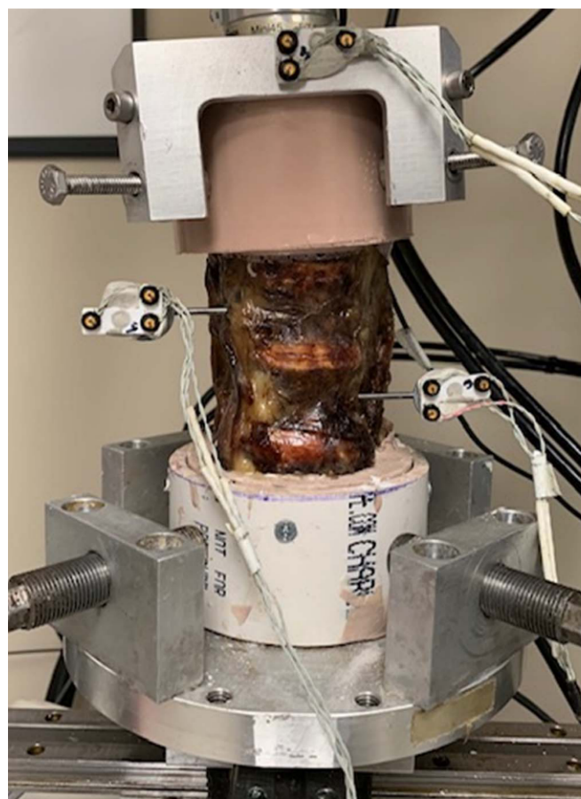
Figure 1. Anterior aspect of a vertebral motion segment mounted in the servohydraulic testing system with optical tracking sensors affixed.
