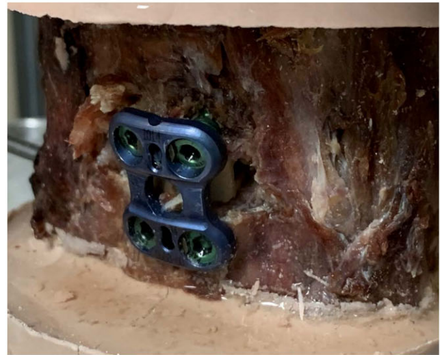
FIGURE 2. Specimen with an anterior cervical plate and interbody spacer (CP) construct, using the RESONATE ® anterior plate and COVERIS ® spacer. full color online
